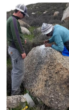
Image 5- Beginning the process of hammering out the sample after making a drill hole for shims and wedges
